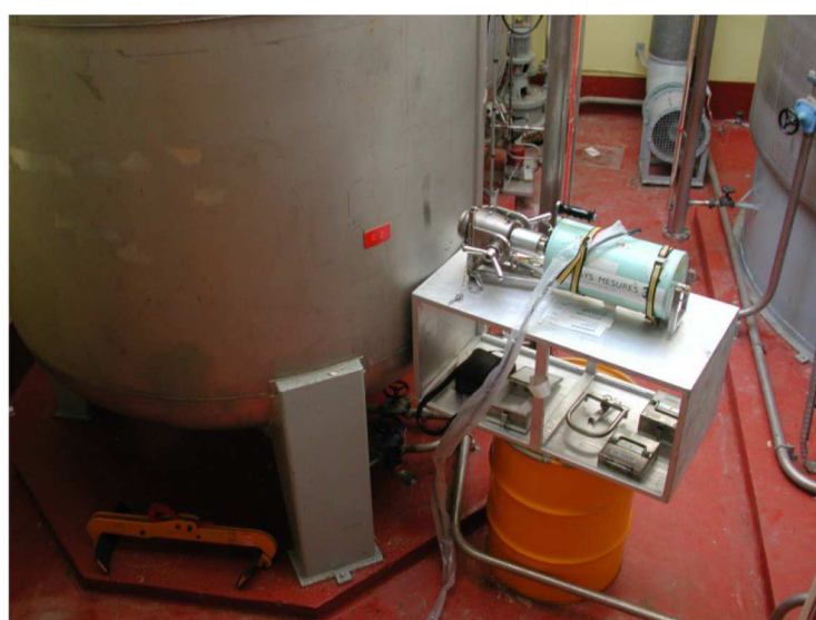
Figure 5: Measurement of a vessel containing radioactive effluents with a collimated HPGe detector (Pérot et al., 2018).
