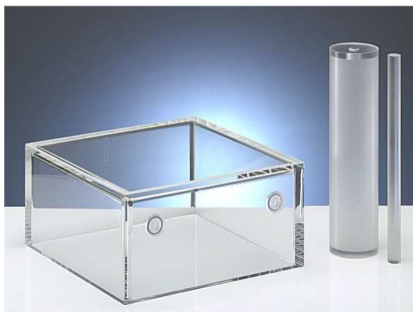
Figure A-3: Phantoms representing parts of human bodies (torso, arm and finger).
