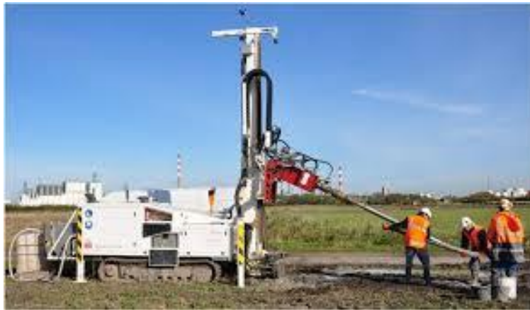
Figure 4: Sonic drilling machine similar to the one used on UC3.
