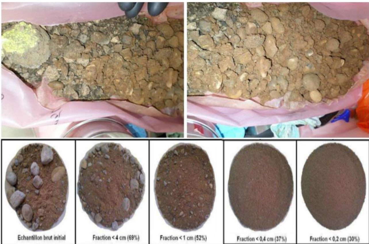
Figure 6: Raw drilling core (top) and result of size segregation (bottom).
